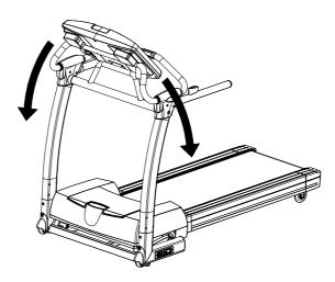
3. Tilt treadmill to access stabilizers.
